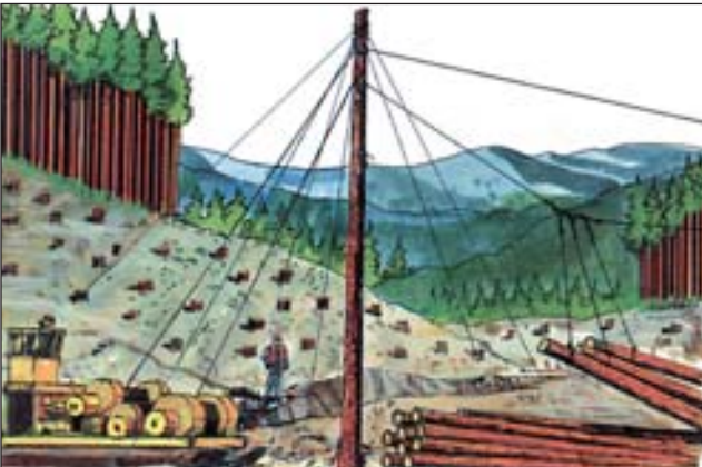
Skid-mounted yarder with wooden spar.
