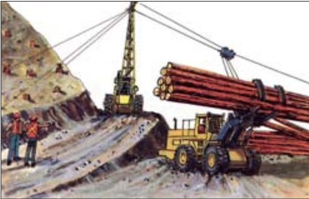
Jump-up landing for a small wood yarder.
