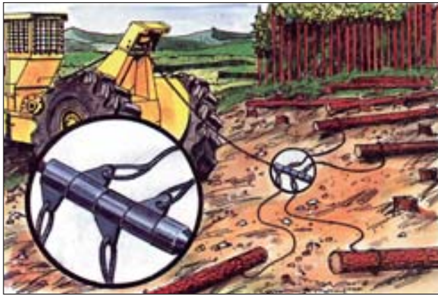
Single drum yarder with multiple chokers attached to the mainline.
