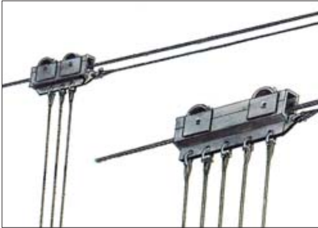
Shotgun carriages with multiple chokers attached.
