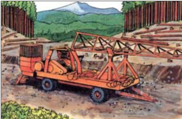
A small trailer-mounted yarder ready for transport.
