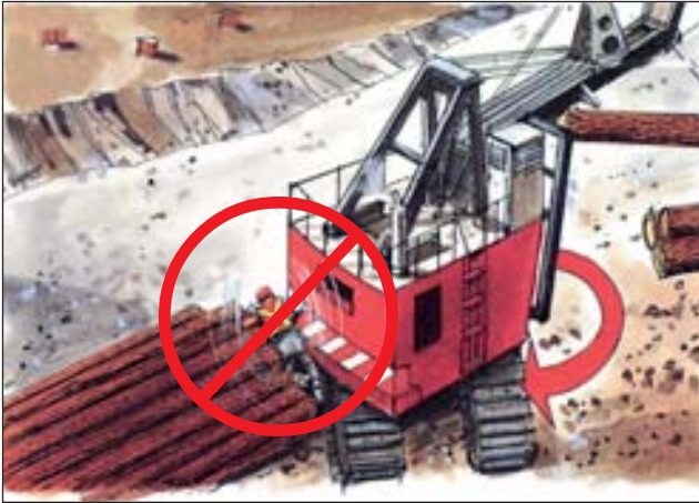
No counterweight clearance.
