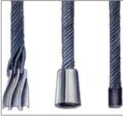
(a) Wedge socket. (b) Pressed ferrule. (c) Whipped end.
