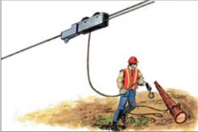
Mechanical stop holding a shotgun carriage.
