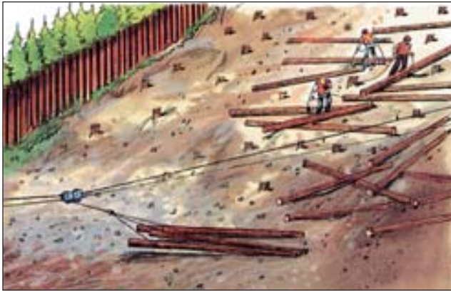
Worker in the clear pre-setting chokers.
