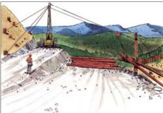
Small wood yarder with intermediate support tree.
