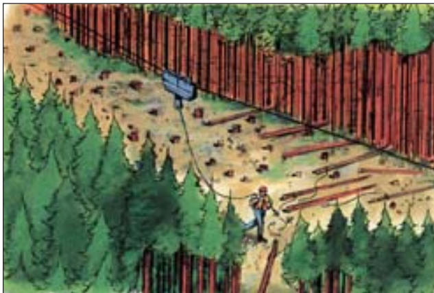
Shotgun system with skyline lock.
