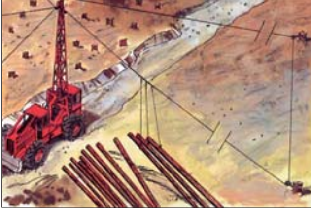
High-lead system on a skidder.
