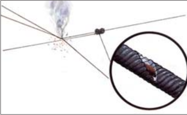
Use of wrong machinery will cause lines to wrap and burn.
