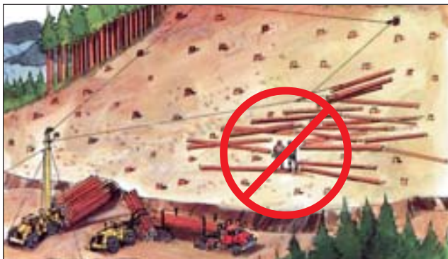
Do not work below log pile during loading.
