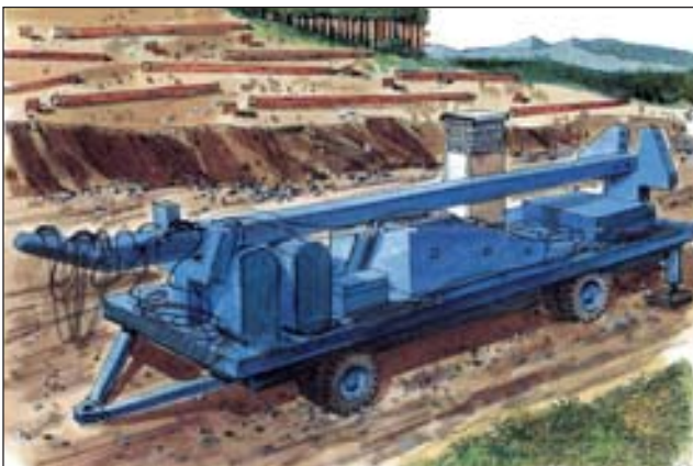
A large trailer-mounted yarder ready for transport.
