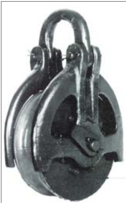
Roller backspar jack with aluminum sheave.
