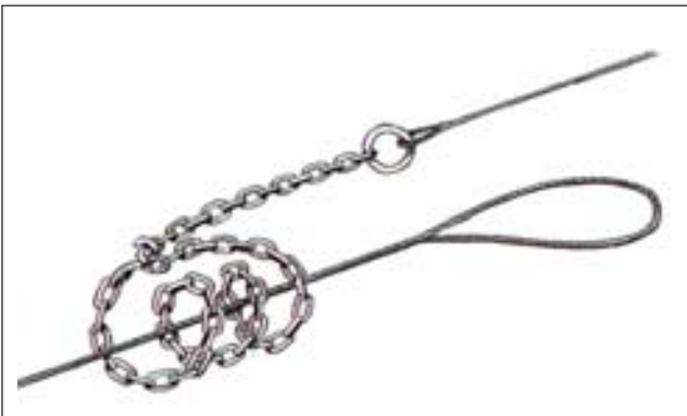
Pass chain wrapped against the pull.
