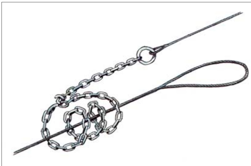
Pass chain wrapped at least three times against the pull.
