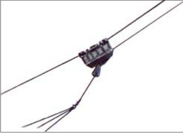
Shotgun carriage with accumulator clamp for downhill yarding.
