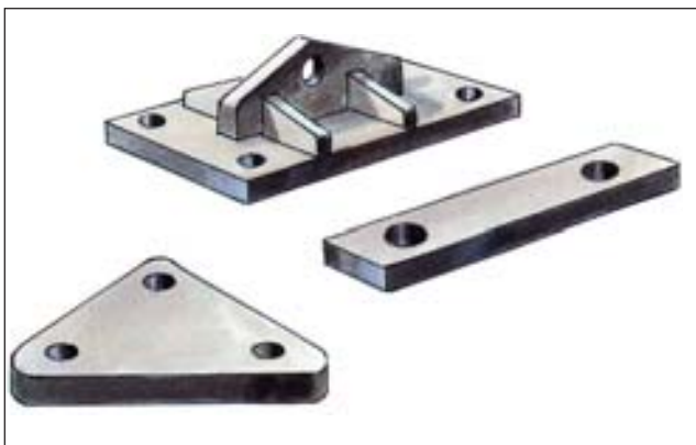
Steel pin plates.
