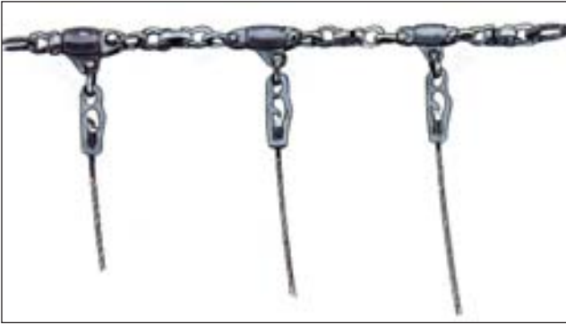
Butt rigging with three chokers.
