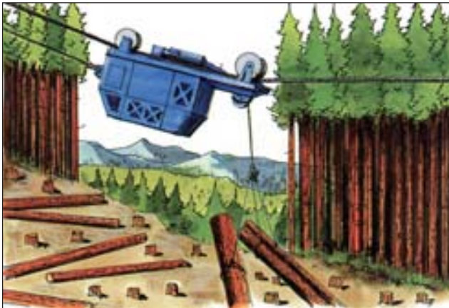
Radio-controlled carriage – no haulback.
