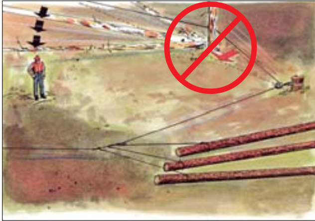
Worker in the bight will be hit by a siwashed line.
