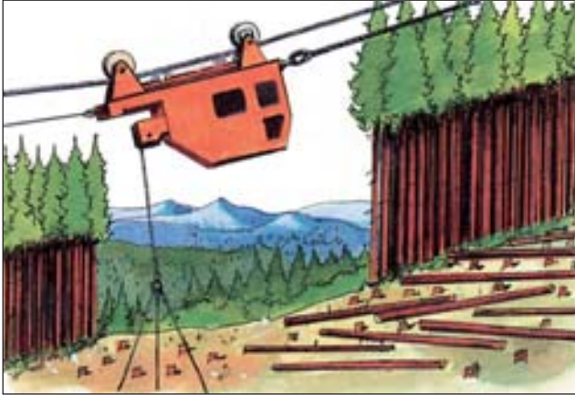
Radio-controlled carriage with haulback attached.
