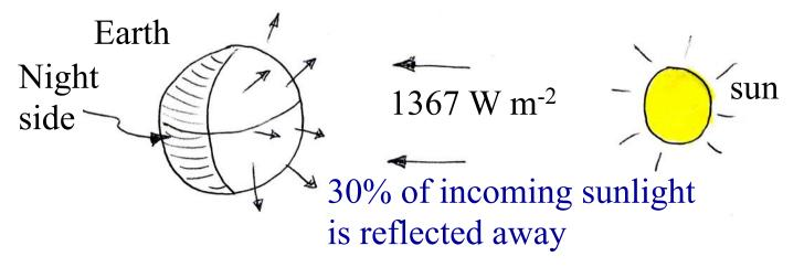
• The remaining energy (70%) must be absorbed by the Earth:  $0.7 \times 342 \text{ W m}^{-2} \approx 240 \text{ W m}^{-2}$
