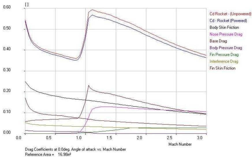
If you can get the rocket higher in altitude before going to high speed, effects from drag can be minimized
