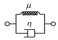
Spring and dashpot together support stress  $\sigma$
