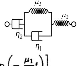
$$e(t) = \frac{\sigma}{\eta_2}t + \frac{\sigma}{\mu_2} + \frac{\sigma}{\mu_1}\left[1 - \exp\left(-\frac{\mu_1}{\eta_1}t\right)\right]$$
