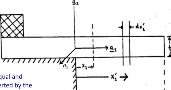
$M_g$  must be balanced by an equal and opposite moment  $M_t$  at  $x_1$  exerted by the stress state there.
