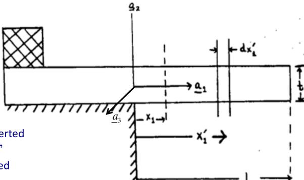
Incremental moment at  $x_1$  exerted by thin slice  $\mathrm{d}x_1$ ' of slab at  $x_1$ ' e.g.  $<\sigma_{12}>$ t is vertically directed force per unit width in  $x_3$
