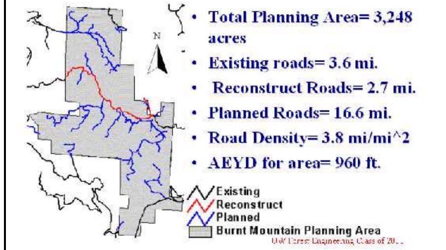
Figure 31 General statistics for all roads in the planning area. Existing roads that require reconstruction are shown in red, other existing road are shown in black. The roads shown in blue are the roads planned for this project (AEYD = average external yarding distance).
