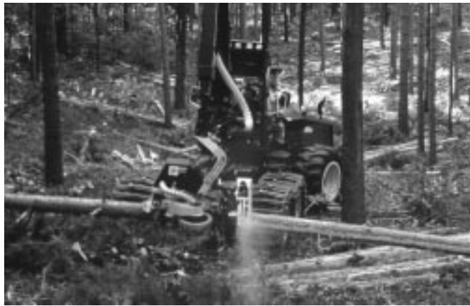
Figure 8 — The typical feller-buncher as used in the Pacific Northwest is track mounted and is designed to work on flat to moderately sloping terrain. Some of these machines have tilting cabs as shown here.
