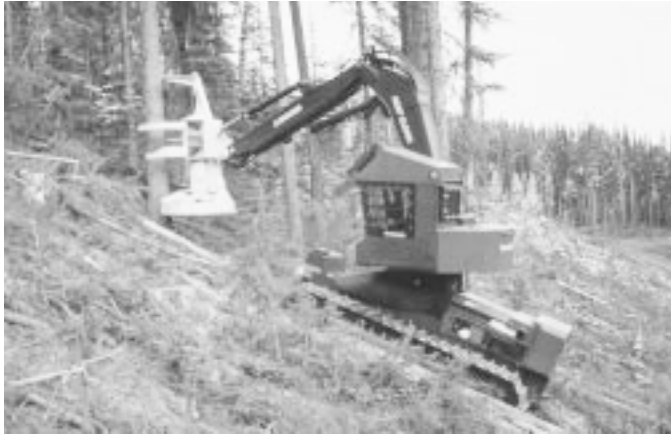
Figure 8 — The typical feller-buncher as used in the Pacific Northwest is track mounted and is designed to work on flat to moderately sloping terrain. Some of these machines have tilting cabs as shown here.
