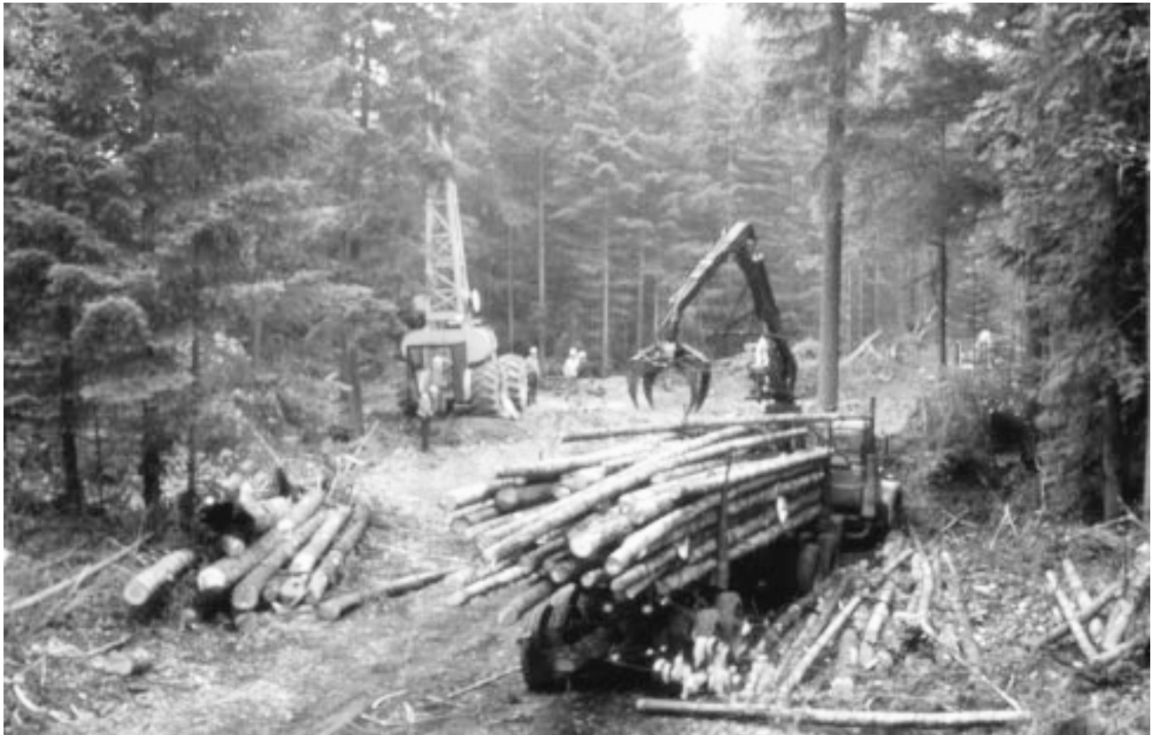
Figure 30 — A self-loading log truck with a hydraulic knuckle boom loader can provide an economic means of delivering small harvest volumes to the mill.
