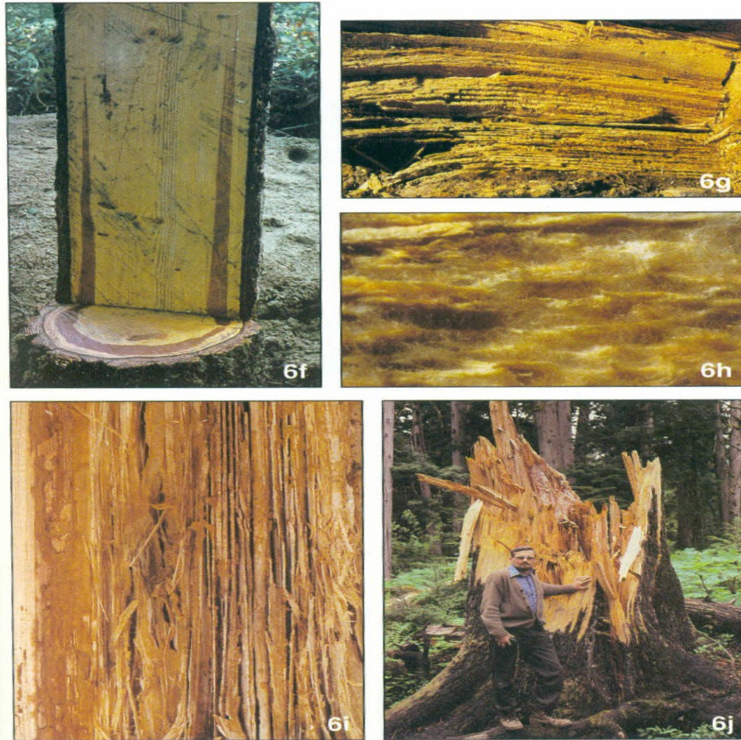
Figure 6f: Incipient decay in outer sapwood of Douglas-fir. Figure 6g: Laminated decay of Douglas-fir typi-
