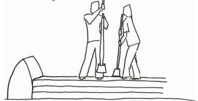
3) Tamp each row and lay barb wire between rows to prevent slipping.
