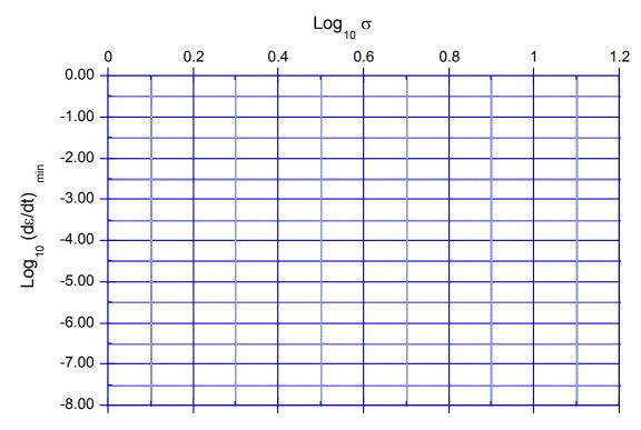
**5)** Determine the slope, m, and intercept, b, of the linear curve fit of the results of the **SHORT TERM** tests **ONLY**. Draw the line on the plot and label the short and long term results. The slope is the stress exponent, n, such that m=n. The intercept, b, is the Log<sub>10</sub> of the pre-exponential constant B such that B=10<sup>b</sup>.
