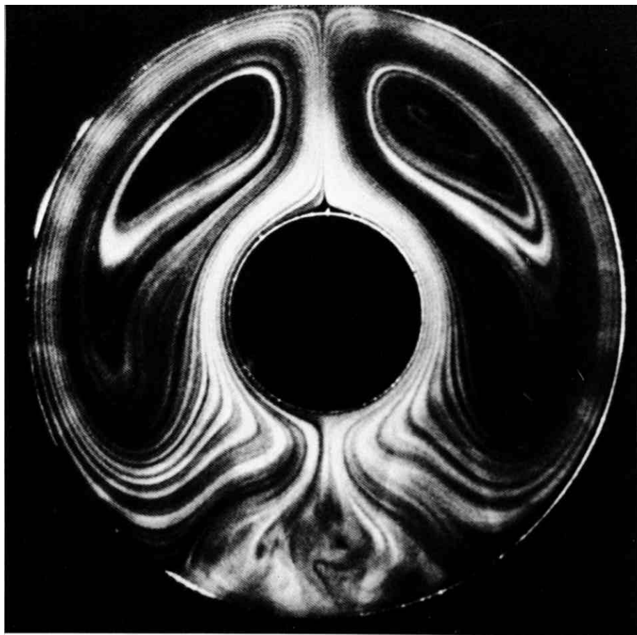
208. Streamlines in convection between concentric cylinders. Cigarette smoke shows the fully developed laminar flow pattern in air at atmospheric pressure. The outer cylinder has three times the diameter of the inner one, and is 14.5^{\circ}\text{C} cooler, giving a Grashof number of 120,000 based on the gap width. Grigull & Hauf 1966
