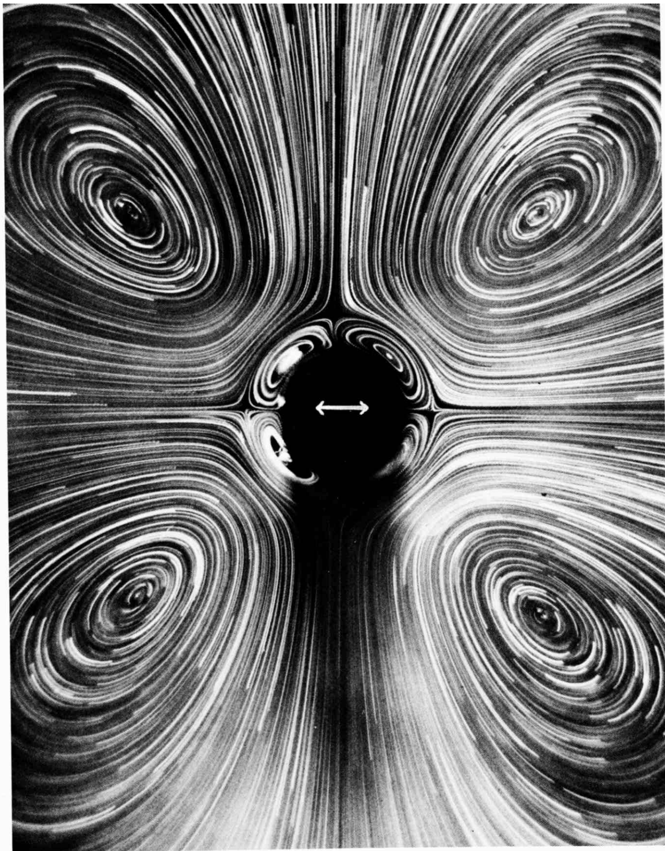
31. Secondary streaming induced by an oscillating cylinder. A long circular cylinder is oscillated normal to its axis by a loudspeaker in a mixture of water and glycerine. Suspended glass beads are illuminated in a cross plane by a stroboscope. The amplitude of oscillation is 0.17 of the
