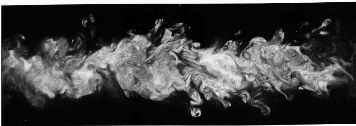
174. Turbulent wake of a cylinder. A sheet of laser light slices through the wake of a circular cylinder at a Reynolds number of 1770. Oil fog shows the instantaneous flow pat-
