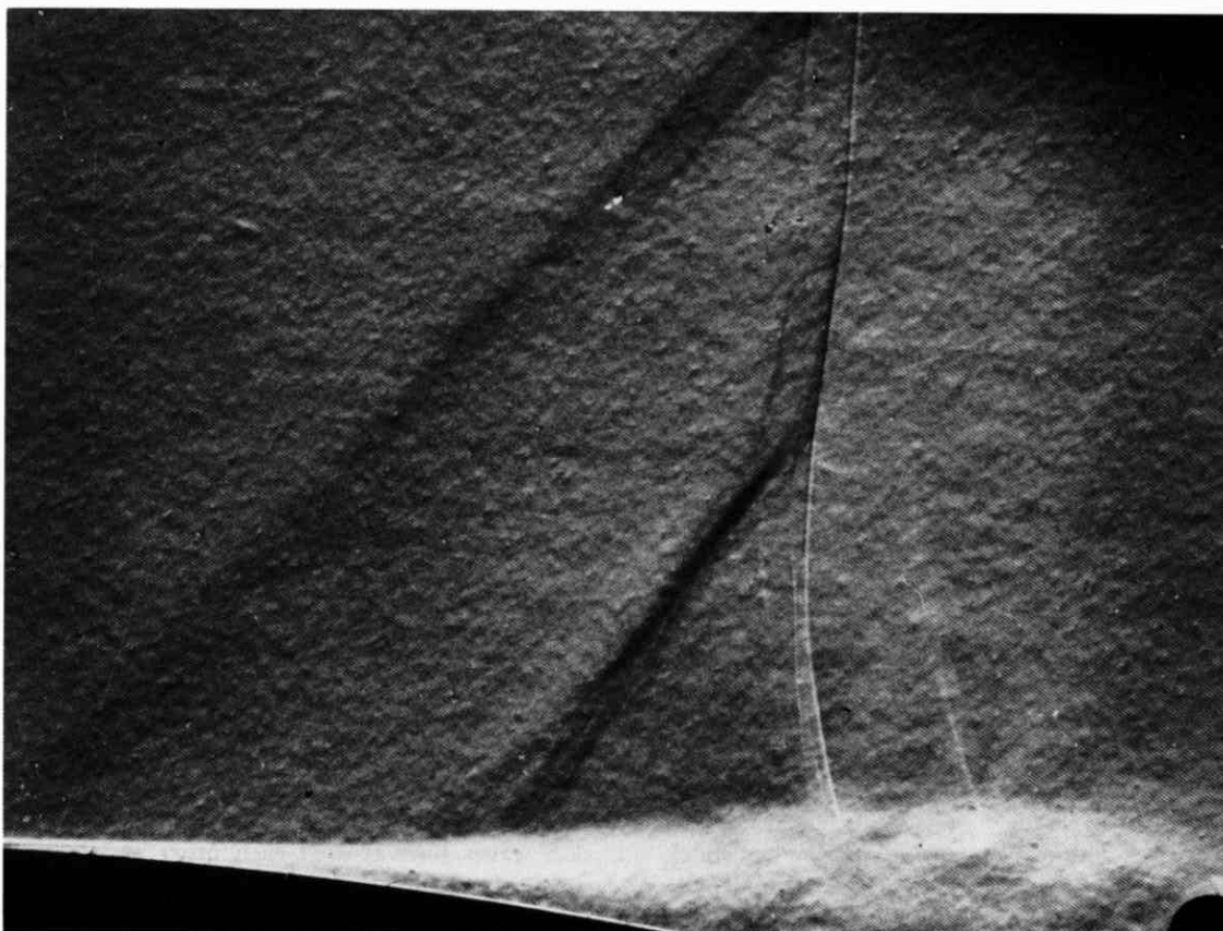
246. Single lambda shock wave on an airfoil with a laminar boundary layer. As the Mach number is increased the multiple shock waves of the upper photograph merge into one. Here a horizontal knife edge shows that at
