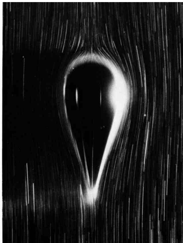
183. Bubble rising in a non-Newtonian fluid. A bubble of 13 \text{ cm}^3 volume rises at a Reynolds number less than 0.1 in a vertical tube of 8.2 cm diameter (not visible) filled with a 3.5 per cent aqueous solution of polyethylene oxide. This fluid possesses both a highly shear-thinning viscosity and considerable elasticity. The bubble loses the fore-aft symmetry it would have in a Newtonian fluid, becoming pointed at the rear. Photograph by M. Coutanceau and P. Thizon, in van Wijngaarden & Vossers 1978
