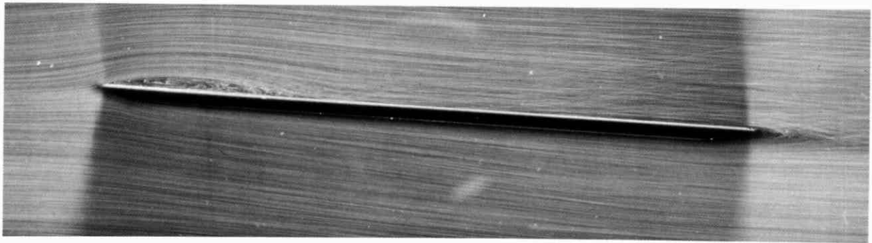
35. Leading-edge separation on a plate with laminar reattachment. A flat plate 2 per cent thick with beveled edges is inclined at 2.5^\circ to the stream. The laminar boundary layer separates at the leading edge over the upper sur-
