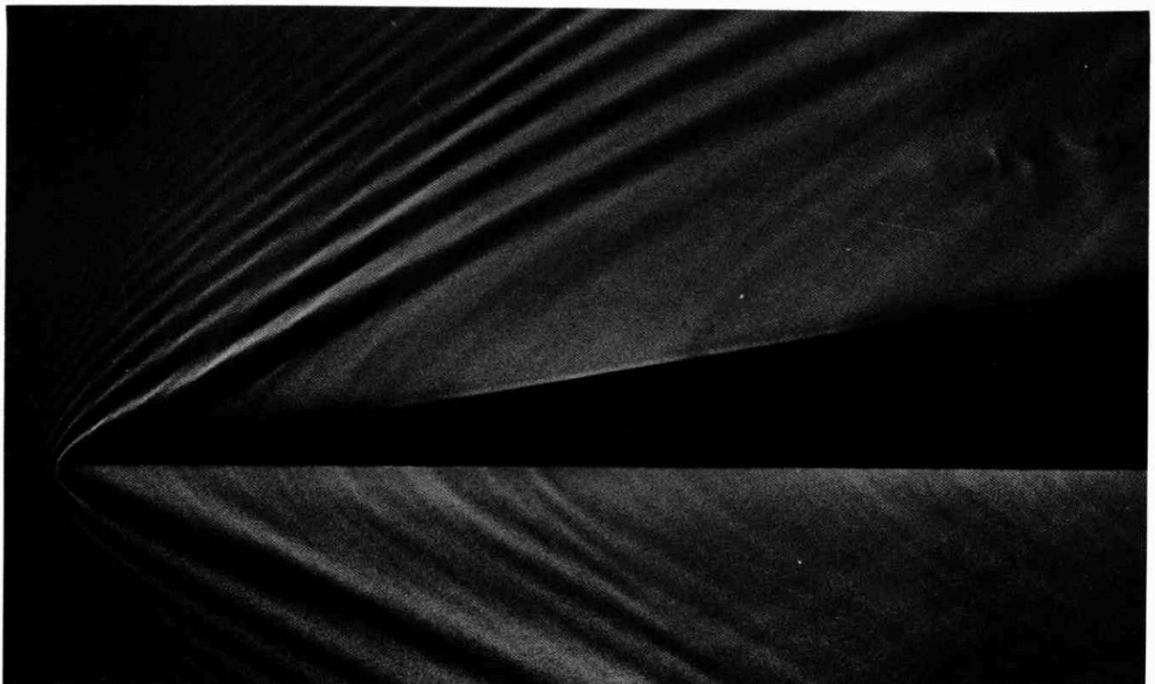
229. Hydraulic analogy for a wedge in supersonic flow. A uniform sheet of water 5 mm deep flows at supercritical speed over a horizontal plane, and is deflected by a sharp 10^\circ wedge with its lower edge parallel to the stream.
