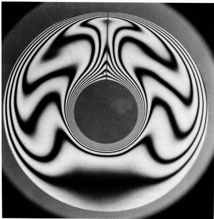
209. Isotherms in convection between concentric cylinders. An interferogram shows the temperature distribution under almost the same conditions as above: ratio of diameters 3.14, temperature difference 13^{\circ}\text{C} , and Grashof number 122,000. Both views show almost stagnant fluid below the inner cylinder. Grigull & Hauf 1966
