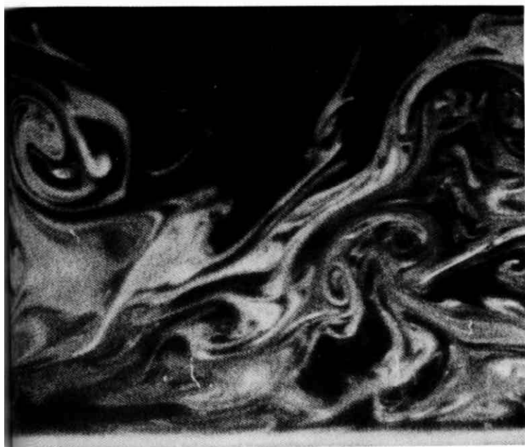
162. "Typical eddy" in a turbulent boundary layer. Oil fog is illuminated by a sheet of laser light to show the lower two-thirds of a turbulent boundary layer in side view. The vortex-ring structure just below and to the right of center, which resembles a sliced mushroom leaning left, is an example of what Falcó has called a "typical eddy." It scales on wall variables (figure 161) rather than on the boundary-layer thickness. Photograph by R. E. Falco
