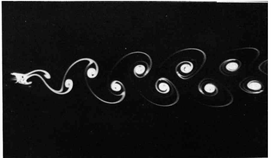
96. Kármán vortex street behind a circular cylinder at R=105 . The initially spreading wake shown opposite develops into the two parallel rows of staggered vortices that von Kármán's inviscid theory shows to be stable when the ratio of width to streamwise spacing is 0.28. Streaklines are shown by electrolytic precipitation in water. Photograph by Sadatoshi Taneda
