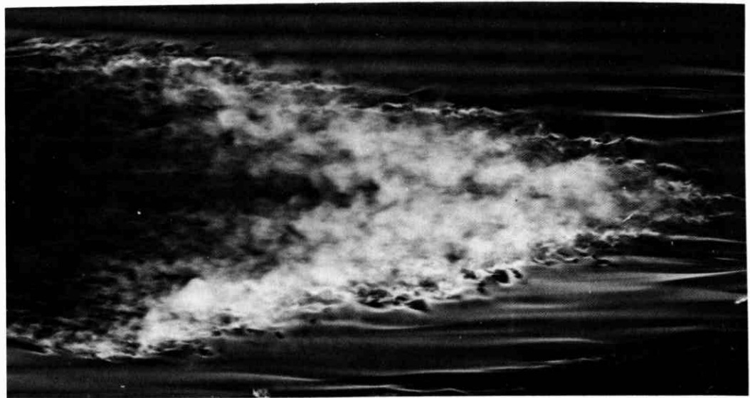
111. Turbulent spot at different Reynolds numbers. The outline of the spot becomes more regular, and the angle of its leading edge steeper, as the Reynolds number
