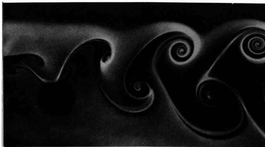
95. Kármán vortex street behind a circular cylinder at R=200 . This photograph, made using a different fluid (and in another country) happens to have been timed so as to resemble remarkably the flow pattern in the upper picture. A thin sheet of tobacco smoke is introduced upstream in a low-turbulence wind tunnel. Photograph by Gary Koopmann
