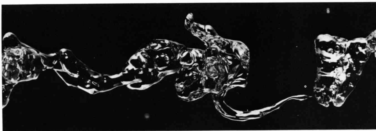
180. Water jet emerging into stagnant air. Water flows at 25 m/s from a nozzle of 6-mm diameter. The jet is seen to be initially laminar, but axisymmetric waves of insta-
