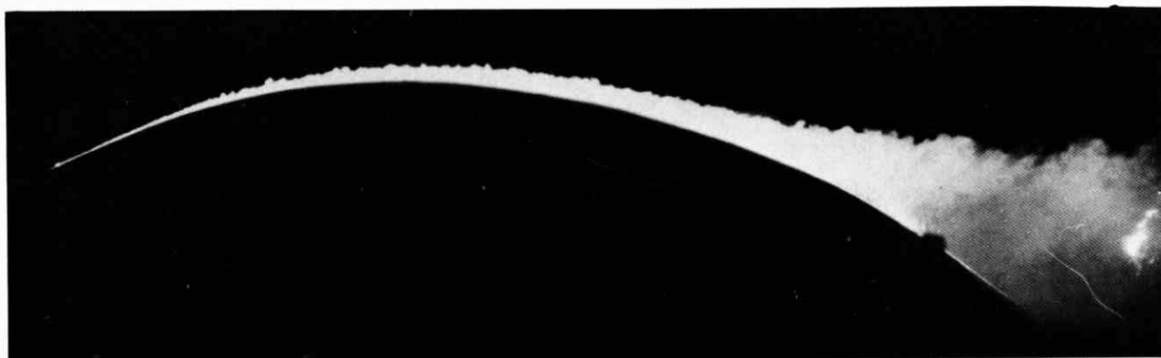
156. Comparison of laminar and turbulent boundary layers. The laminar boundary layer in the upper photograph separates from the crest of a convex surface (cf. figure 38), whereas the turbulent layer in the second
