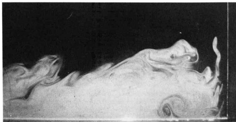
165. Turbulent boundary layer encountering a cylinder. As the turbulent boundary layer flows around a circular cylinder normal to the wall, eddies in the outer region are rapidly distorted and an intermittent reversed jet forms in the separated region. Figure 92 shows the corresponding flow with a laminar boundary layer. Photograph by R. E. Falco
