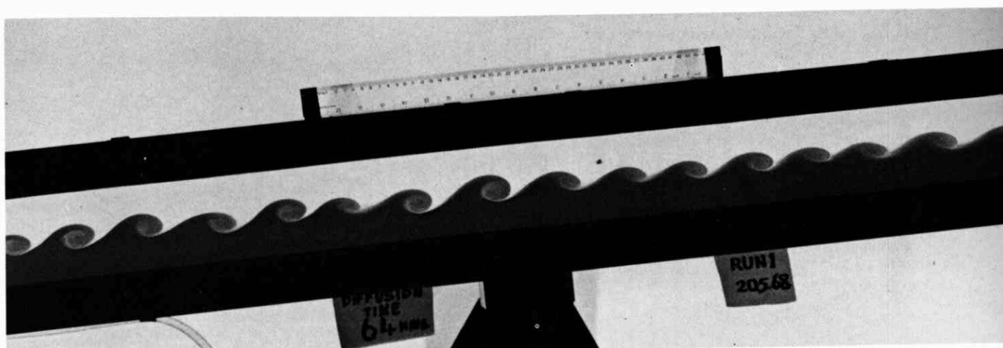
145. Kelvin-Helmholtz instability of stratified shear flow. A long rectangular tube, initially horizontal, is filled with water above colored brine. The fluids are allowed to diffuse for about an hour, and the tube then quickly tilted six degrees, setting the fluids into motion. The brine accel-
