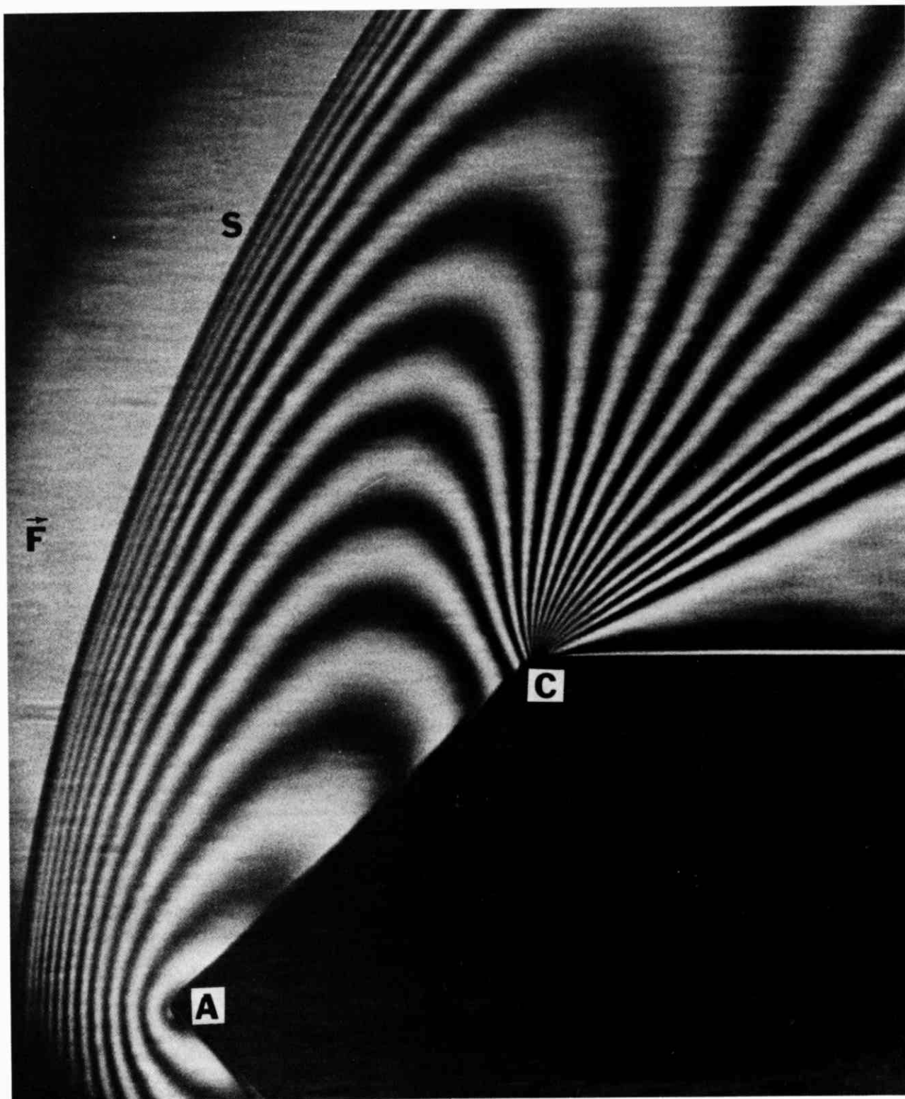
234. Detached bow shock wave on a thick wedge. An infinite-fringe interferogram shows lines of constant density about a wedge A of 45^\circ half angle in a stream of air F at Mach number 2.5. No attached shock wave can turn the
