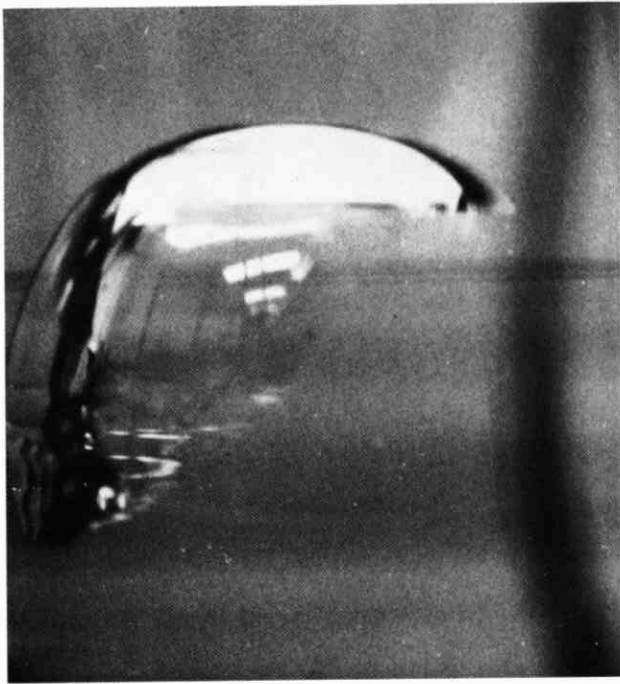
185. Spherical-cap bubbles with "skirts." Bubbles containing 50-100 cm 3 of air are rising in mineral oil. For speeds above some 40 cm/s and viscosities above 200 centi-
