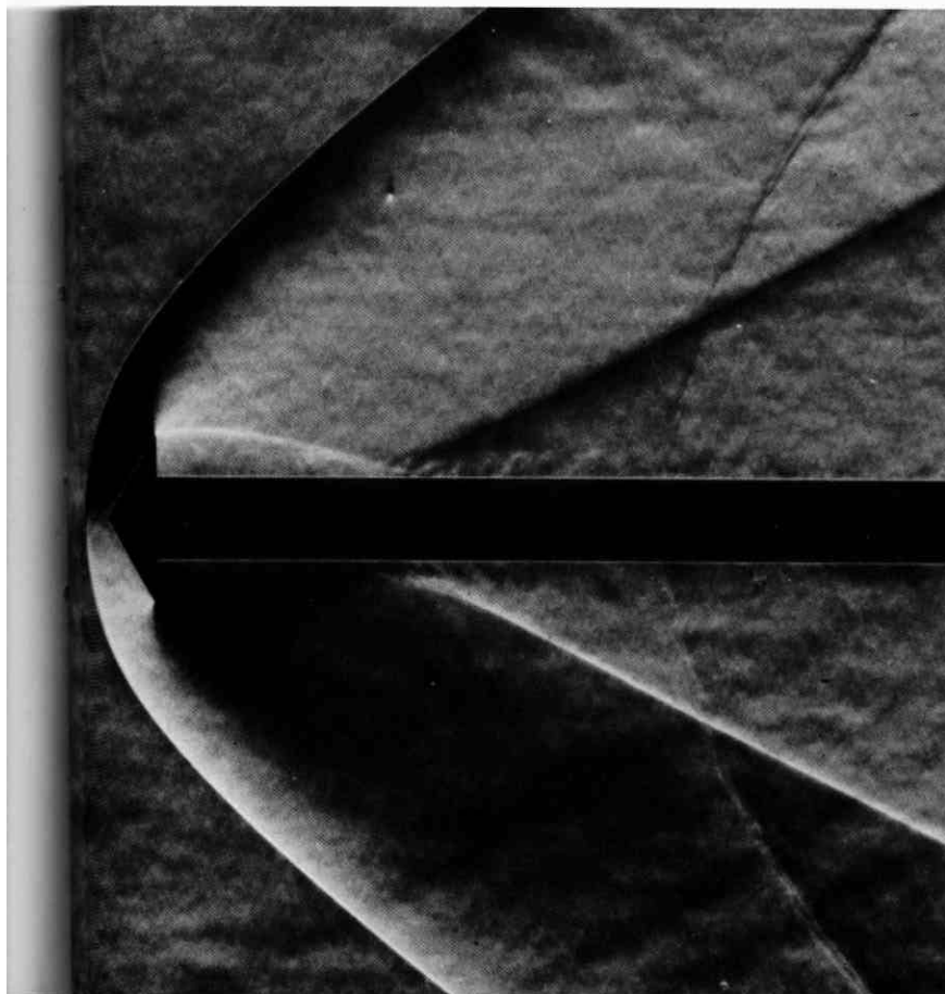
258. Detached bow wave on a 60^\circ cone at M=1.96 . At this Mach number in air the bow shock wave cannot remain attached to the vertex of a cone above a semi-vertex angle of 40^\circ . It detaches, forming an embedded subsonic zone extending back to the cone surface. The two crinkled curves downstream are the intersections of the bow wave with the turbulent boundary layers on the wind-tunnel windows. Photograph by A. W. Sharp, courtesy of N. Johannesen
