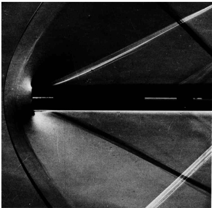
262. Flat-faced plate at M=2.0 . The knife edge is horizontal in this schlieren photograph, so that light above is dark below. Gaps in the middle of the plate do not affect the air flow. The curved line just downstream of the detached bow shock wave is caused by its intersection with the boundary layers on the glass sides of the wind tunnel. The boundary layer separates at the corner, and its reattachment is marked by the formation of oblique shock waves. Mair 1952, courtesy of N. Johannesen
