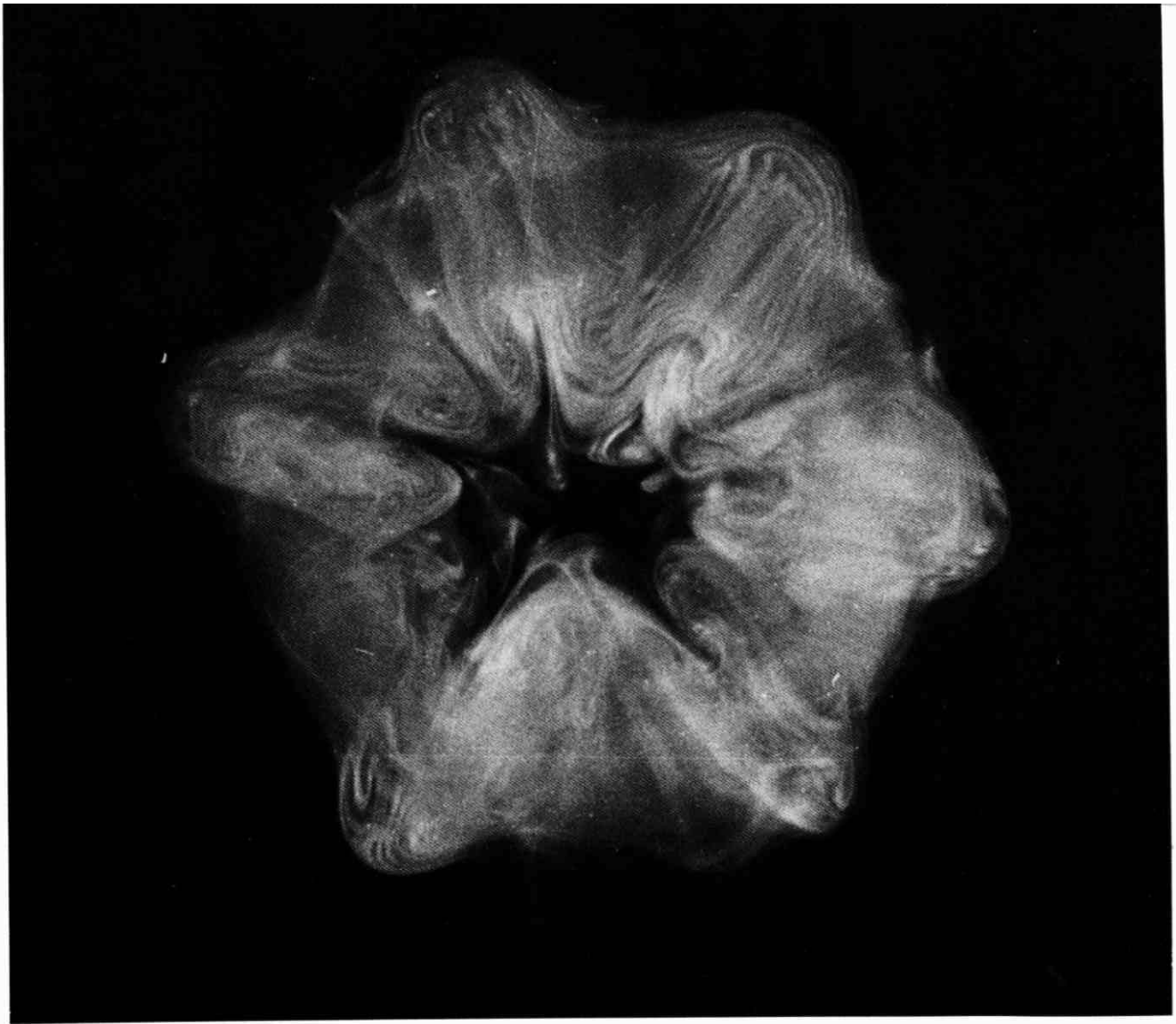
113. Hexagonal smoke ring. The growth of waves around a vortex ring is often called Widnall instability, after the researcher who first analyzed it. Here it has pro-
