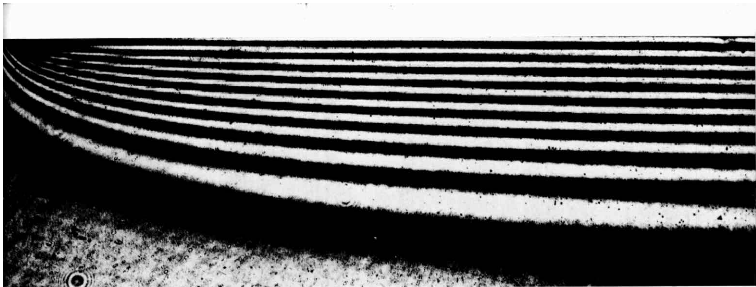
210. Thermal boundary layer beneath a horizontal plate. A laser-holographic interferogram shows isotherms in air, averaged over a 30-cm depth, under the left half of a heated rectangular aluminum plate 10 cm wide and 1 cm thick. The edge of the plate lies directly above the small
