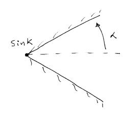
The potential (inviscid, irrotational) approximation is valid away from the walls and predict a velocity field:  $V_r(r) = \frac{m}{2\pi e r}$   $V_0 = 0$ Applying Bernouilli to the potential flow velocity.  $P(r) + \frac{1}{2} S V^2 = P_{ro} + \frac{1}{2} S V_{ro}^2$   $P(r) = \left[P_{ro} + \frac{1}{2} S \left(V_{ro}^2 - \frac{m^2}{4\pi^2 e^2 r^2}\right)\right]$
