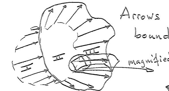
Arrows are the local velocity at the boundary of the volume at  $t=t_0$ .
