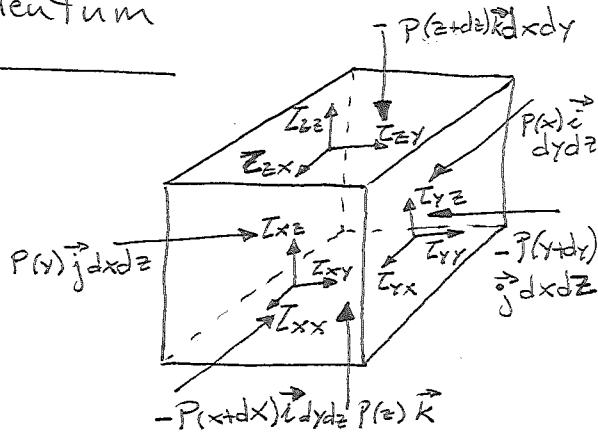
$$\frac{\partial}{\partial t} \int_{C.V.} \rho \vec{v} dV + \int_{C.S.} \rho \vec{v} (\vec{v} - \vec{v}_0) \cdot \vec{n} dA = - \int_{C.S.} p \vec{n} dA + \int_{C.S.} \vec{F} \cdot \vec{n} dA + \int_{C.V.} \vec{G} \cdot \vec{n} dV$$
