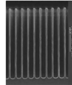
cross section of a silicon wafer demonstrating trenches that can be fabricated using DRIE tech
