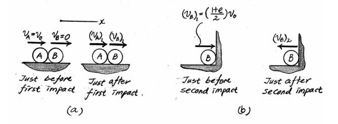
Disks A and B have a mass of 15 kg and 10 kg, respectively. If they are sliding on a smooth horizontal plane with the velocities shown, determine their speeds just after impact. The coefficient of restitution between them is e = 0.8.
