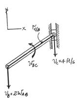
If the flywheel is rotating with an angular velocity of  $\omega_A = 6$  rad/s, determine the angular velocity of rod BC at the instant shown.
