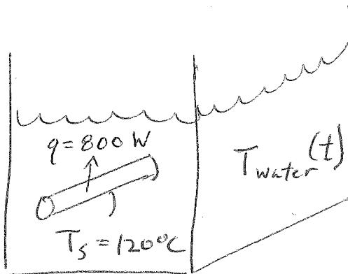
Control Volume is around the water, excluding the electric resistance heater.
