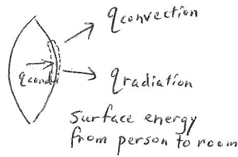
Assumptions: For gray surface,  $\epsilon_{\text{person}} = 0.90$ , in a large enclosure,  $q_{\text{radiation}} = \epsilon \sigma A (T_s^4 - T_{\text{surr}}^4)$
