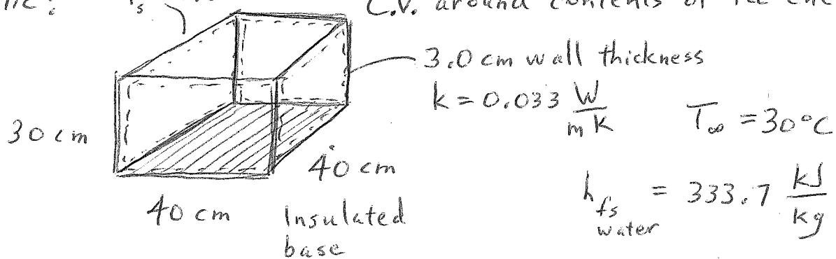
Assumptions: Inner surfaces of ice chest are at uniform temperature  $0.0^\circ\text{C}$ . Outer surfaces of top and four side walls are at uniform temperature  $8.0^\circ\text{C}$ . 1-D conduction is assumed through these five walls. Base of ice chest is insulated. No sensible energy change.
