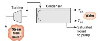
(a) If cooling water from a large lake is pumped through the condenser tubes at  $\dot{m}_c = 400$  kg/s, what is the overall heat transfer coefficient  $U_o$  based on the outer surface area of a tube? Water properties may be approximated as  $\mu = 9.60 \times 10^{-4}$  N-s/m<sup>2</sup>, k = 0.60 W/m-K, and Pr = 6.6. (b) If after extended operation, fouling provides a resistance of  $R''_{f,l} = 10^{-4}$  m<sup>2</sup>-K/W, at the inner surface, what is the value of  $U_o$ ?
