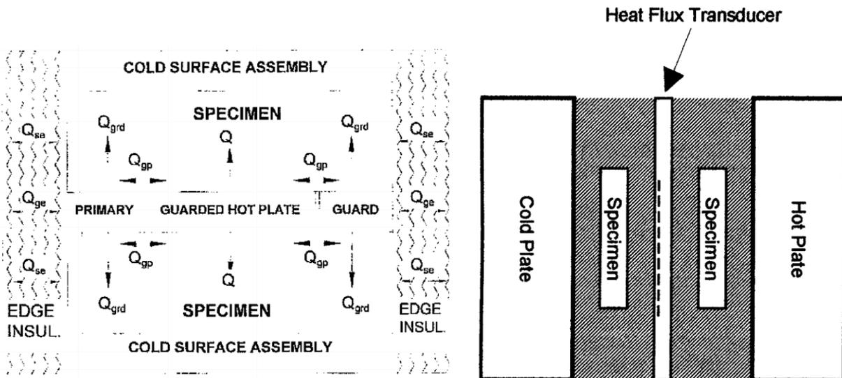
Figure 2. Idealized heat flow for ASTM-C-177 test apparatus (left) [4]. ASTM-C-518 test apparatus (right) [3].
