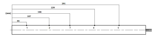
The thermocouples are Type K, chromel-alumel, made from 30 gauge wire. As shown in the figure above, thermocouples 1 through 5 are mounted at the specified distances in mm from the end of the rod heater. Likewise, thermocouples o1 through o5 are respectively mounted at these same axial distances on the outer surface of the tubular insulation material.
