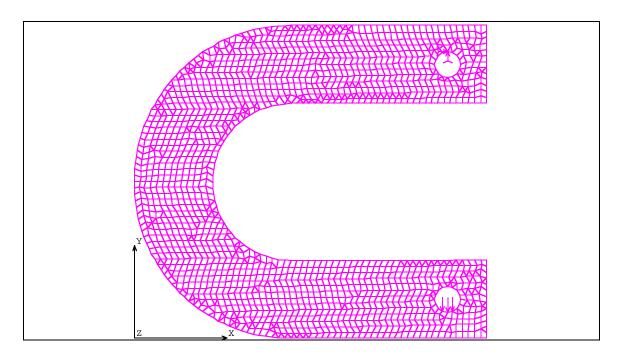
Plane stress two-dimensional model: 1787 elements (both quadrilateral and triangular) and 1350 nodes. Nodal loading and constraints at the pin holes.
