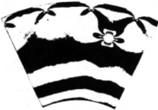
Fig. 6.26. Isochromatic pattern for central slice.
