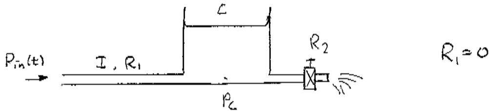
$$P_c(t) = \bar{P}_c + \Delta P_c(t), \quad P_{in}(t) = \bar{P}_{in} + \Delta P_{in}(t)$$
