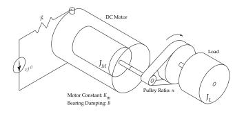
A belt and pulley connect the motor to the rotational load. The parameter values are:
