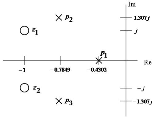
Figure 4: Fluid system poles and zeros
