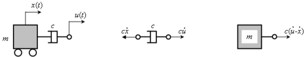
Figure 1: Mass-damper system; free-body diagrams
