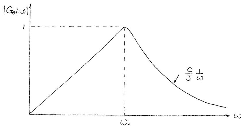
(c) To measure  $\Omega_s(t)$ , we should use  $T_k$  as output, because when  $\omega \ll \omega_n$   $|G_k(\omega)|$  will be in a flat zone. The bandwidth of tachometer is  $\omega_c$ . The sensitivity is constant for  $|G_k(\omega)|$  flat zone, which is  $c$ .
