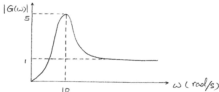
$$\left. \begin{aligned} |G_u(\omega)| &= \frac{m\omega^2}{\sqrt{(k - m\omega^2)^2 + c^2\omega^2}} \\ \zeta &= \frac{c}{2m\omega_n} \Rightarrow c = 2\zeta m\omega_n \end{aligned} \right\}$$
