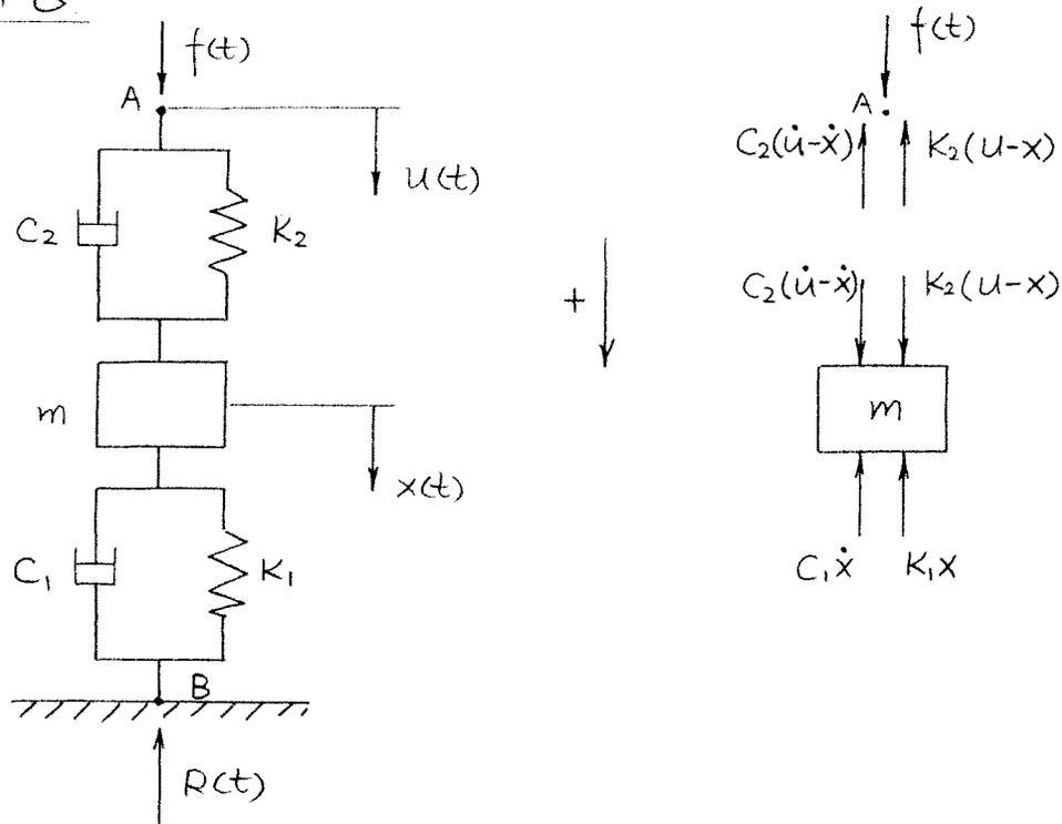
(a) Point A:  $\Sigma F: f(t) - C_2(\dot{u} - \dot{x}) - K_2(u - x) = 0$
