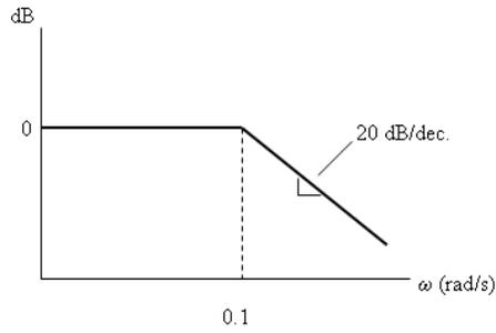
Figure 1: Magnitude of the frequency response function  $G(\omega)$ .
