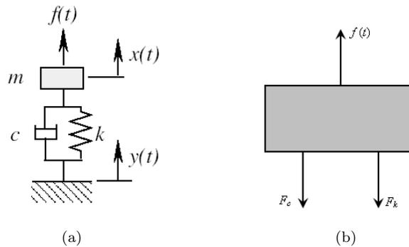
Figure 5: (a) Model for vibration control; (b) Free-body diagram.
