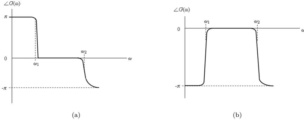
Figure 13: (a) Phase of  $G(\omega)$ ; (b) Alternative phase plot where  $\angle G(\omega \ll \omega_1) = -\pi$ .
