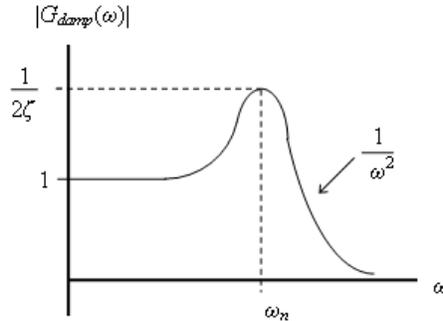
Figure 8: Amplitude of  $G_{damp}(\omega)$ .
