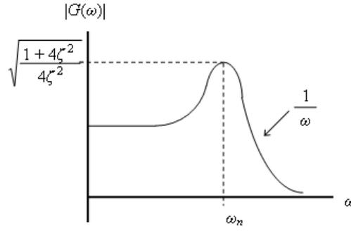
Figure 6: Amplitude of  $G(\omega)$ .
