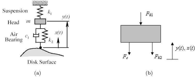
Figure 10: (a) Suspension model in HDD; (b) Free-body diagram of recording head.
