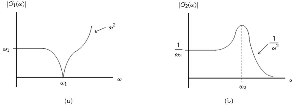
Figure 11: (a) Amplitude of  $G_1(\omega)$ ; (b) Amplitude of  $G_2(\omega)$ .
