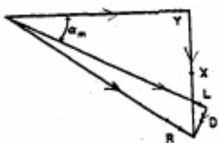
$c_m = c_x / \cos a_m$ . Referring to unit depth (span) of blade, the lift force  $L$  acting on the blade is perpendicular to  $c_m$  and the drag force  $D$  acting on the blade is parallel to  $c_m$ . The resultant force  $R$  has components  $X$  and  $Y$
