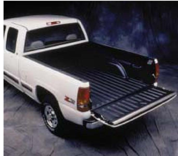
P4-SRIM truck bed and tailgate on 2001 Chevy Silverado is 50 lb and 15 lbf lighter, respectively, than steel counterparts
