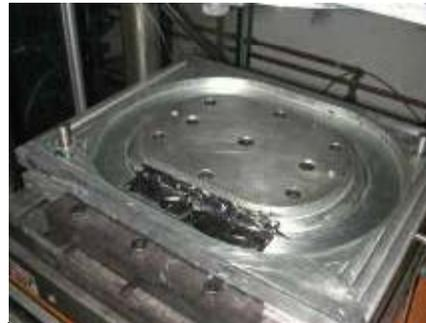
Lay-in L-shaped Front and Back Rib Plies
