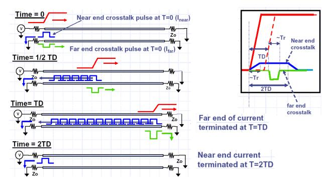
Equivalent circuit model for crosstalk analysis in multiple traces
