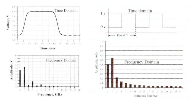
Example: 'Square wave' signal => odd harmonics  $x(t) = \frac{4}{\pi} \left( \sin\left(2\pi ft\right) + \frac{1}{3}\sin\left(2\pi 3ft\right) + \frac{1}{5}\sin\left(2\pi 5ft\right) + \dots \right)$
