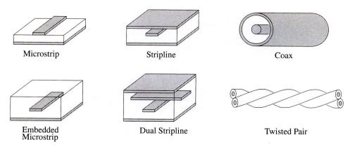
Transmission line is used to transport a signal from one point to another Important parameters
