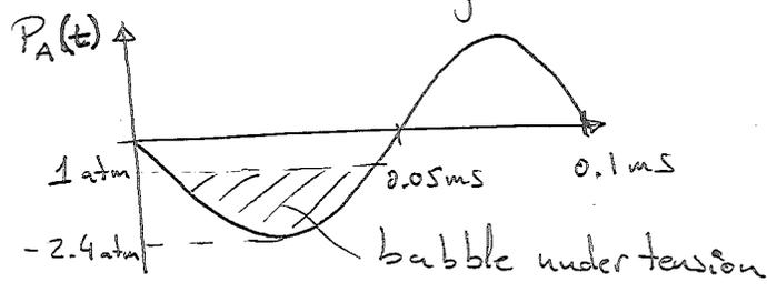
By the time the pressure becomes compressional, the bubble has grown to a really large diameter, creating a very low pressure inside so that the bubble collapses violently due to its own internal depression as much as the external compression.
