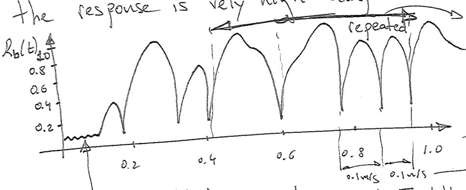
initial oscillations at around 70 kHz (period of 0.014 ms), twice the bubble resonant frequency.
