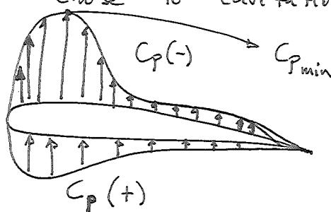
Ideally cavitation would occur at  $\bar{r} = \bar{r}_i^{\text{cav}}$  critical value for inception at the point where  $C_p = C_{p\min}$
