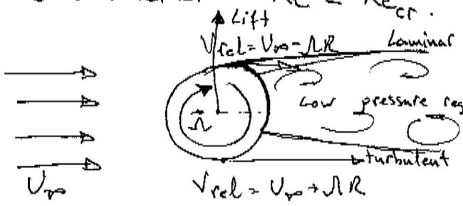
if  $Re < Re_{cr}$  but close to it, the b.l. in the lower half of the sphere may become turbulent, therefore delays separation. The upper half is laminar and separates earlier.
