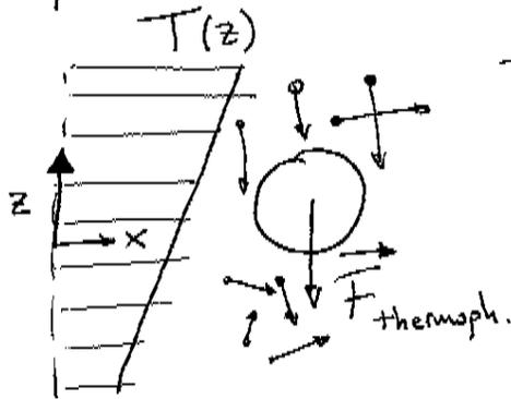
Temperature is a measure of the fluctuating kinetic energy of molecules in a fluid. The larger the temperature the more energy the molecules have and the more momentum they will exchange with particle through collisions.
