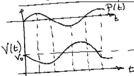
$$P = P_0 + \text{Re} [P^* \sin(kx) e^{i\omega t}]; \quad R = R_0 [1 + \text{Re}(\psi e^{i\omega t})]$$
