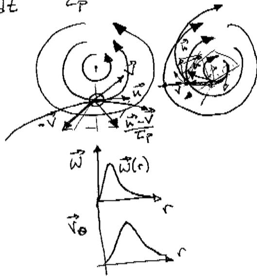
The difference between  $\vec{u}$  and  $\vec{V}$  yield a force that centrifuges the particle out of the core of the vortices "Preferential concentration of particles"
