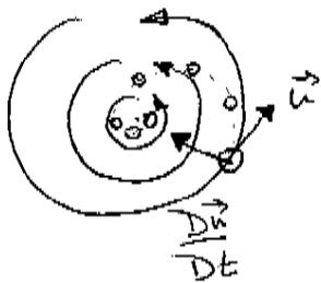
If gravity is acting, bubbles will spend more time on the downward side of eddies than on the upward side, therefore rise velocity will be slower.
