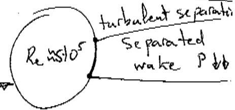
As the Reynolds number increases, the separation point moves upstream, assuming the b.l. is turbulent
