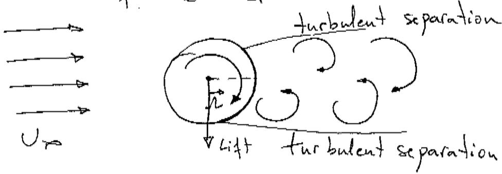
For supercritical conditions, the b.l. is turbulent on both the lower and upper spherical caps and separation occurs <sup>earlier</sup> on the lower half where the relative velocity is higher
