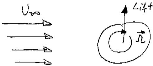
$$\vec{L} = \frac{\pi}{8} D^3 \rho \left[ \left( \frac{1}{2} v_n \vec{u} - \vec{R} \right) \wedge (\vec{u} - \vec{v}) \right]$$
