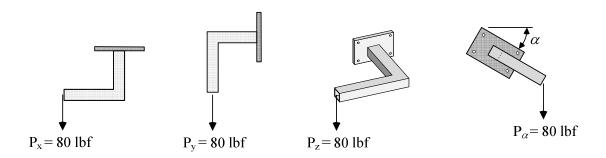
In all cases the load cell will be mounted to the wall pillar plate by means of four bolts, and two 40 lb<sub>f</sub> weights (80 lb<sub>f</sub> total) will be applied to the load cell. The objective of the experiment is to (a) determine the calibration matrix for the load cell (defined in the following discussion), and (b) determine the angle  $\alpha$  associated with the fourth test.
