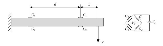
Since the beam has rectangular cross-section, then strains induced at gages  $G_1$  and  $G_2$  are equal in magnitude but opposite in algebraic sign. These strains are due to the bending moment induced at distance x from the transverse force F. Let the strains at gage sites 1 and 2 be given by:
