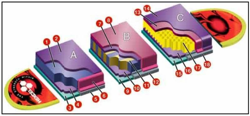
1 Honeycomb/ Polyurethane core 2 Epoxy/Glass, Carbon or Hybrid Top Laminate 3 PE Running Surface: 4 Epoxy/Glass, Carbon or Hybrid Bottom Laminate: 5 Profile Steel Edge: 6 Sidewall (ABS): 7 Top Laminate 8 Decorative Thermoplastic Cap Foil 9 PE Running Surface: www.hexcel.com
