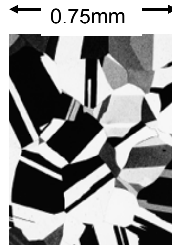
Micrograph of brass (a Cu-Zn alloy)
