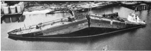
Ship-cyclic loading from waves.
