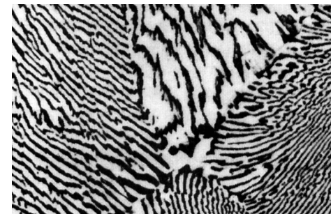
Micrograph of Pb-Sn eutectic microstructure
