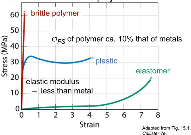
Strains – deformations > 1000% possible (for metals, maximum strain ca. 10% or less)
