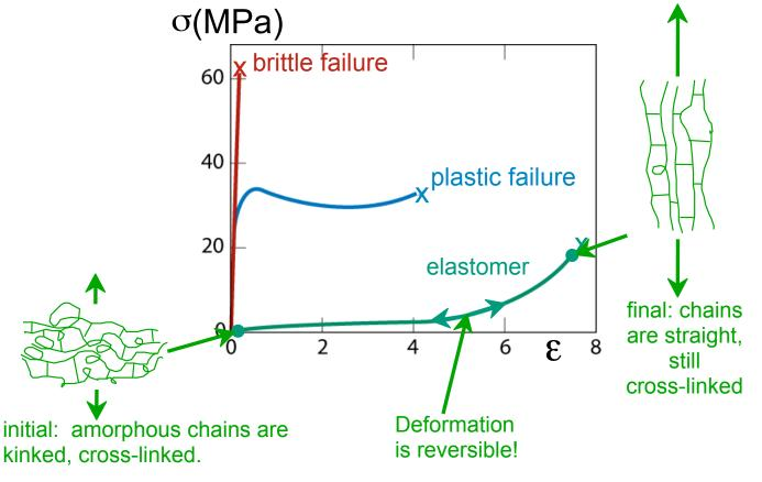
Stress-strain curves adapted from Fig. 15.1, Callister 7e. Inset figures along elastomer curve (green) adapted from Fig. 15.15, Callister 7e. (Fig. 15.15 is from Z.D. Jastrzebski, The Nature and Properties of Engineering Materials, 3rd ed., John Wiley and Sons, 1987.)
