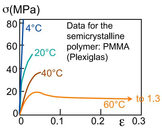
Adapted from Fig. 15.3, *Callister 7e.* (Fig. 15.3 is from T.S. Carswell and J.K. Nason, 'Effect of Environmental Conditions on the Mechanical Properties of Organic Plastics", *Symposium on Plastics*, American Society for Testing and Materials, Philadelphia, PA, 1944.)
