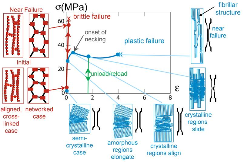
Stress-strain curves adapted from Fig. 15.1, *Callister 7e.* Inset figures along plastic response curve adapted from Figs. 15.12 & 15.13, *Callister 7e.* (Figs. 15.12 & 15.13 are from J.M. Schultz, *Polymer Materials Science*, Prentice-Hall, Inc., 1974, pp. 500-501.)
