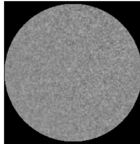
Reprinted with permission from: A.K. Schmid, N.C. Bartelt, and R.Q. Hwang, "Alloying at Surfaces by the Migration of Reactive Two-Dimensional Islands", *Science*, Vol. 290, No. 5496, pp. 1561-64 (2000). Field of view is 1.5  $\mu\text{m}$  and the temperature is 290K.
