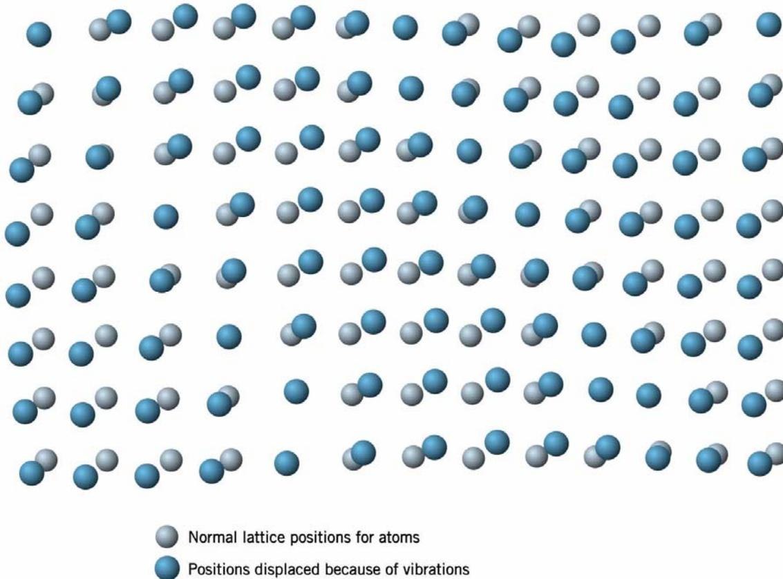
Lattice vibration is a mode of heat transfer through a crystal
