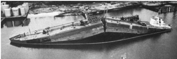
Ship-cyclic loading from waves.
