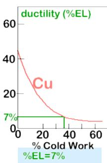
Adapted from Fig. 7.17, *Callister 6e.* (Fig. 7.17 is adapted from *Metals Handbook: Properties and Selection: Iron and Steels*, Vol. 1, 9th ed., B. Bardes (Ed.), American Society for Metals, 1978, p. 226; and *Metals Handbook: Properties and Selection: Nonferrous Alloys and Pure Metals*, Vol. 2, 9th ed., H. Baker (Managing Ed.), American Society for Metals, 1979, p. 276 and 327.)
