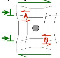
Impurity generates local shear at A and B that opposes disl motion to the right.
