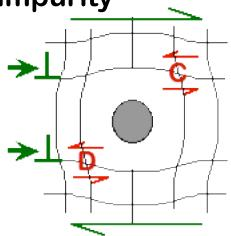
Impurity generates local shear at C and D that opposes disl motion to the right.
