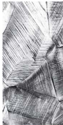
Slip lines on the surface of a polycrystalline specimen of copper
