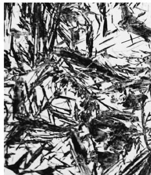
Plate martensitic microstructure
