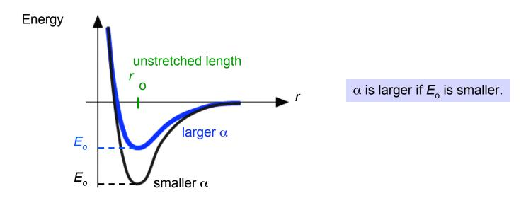
Properties from bonding: modulus *E*
