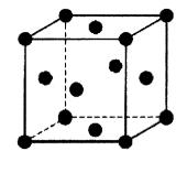
b. Determine the number of atoms per unit cell for the face centered cubic (FCC) structure.
