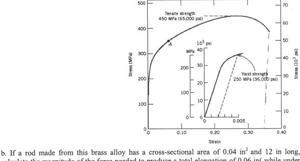
calculate the magnitude of the force needed to produce a total elongation of 0.06 in( while under the load):
