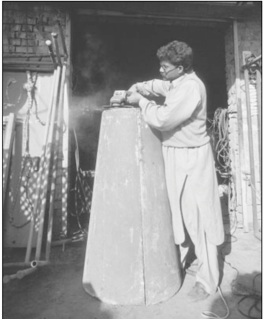
A metal worker makes steel shuttering for a drain manhole in Hassanpura, Faisalabad.
