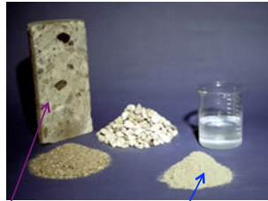
Concrete components: cement, water, fine aggregate (sand), & coarse aggregate (gravel or crushed stone)
