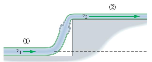
1. Water (assume it is incompressible and non-viscous) flows in a pipe as shown above. The pipe is horizontal at point 1, then rises in elevation while decreasing in diameter and is again horizontal at point 2. Which of the following statements is correct?
