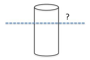
2. A spar buoy consists of a circular cylinder, which floats with its axis oriented vertically. It has a radius of 1.00 m, a height of 2.00 m and weighs 40.0 kN. What portion of it is submerged when it is floating in fresh water?
